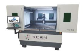
at the front and back as well as side sliding windows make part loading and removal an easy task. SigmaNest® Techno™ software is optional with the FiberCELL system. This advanced CNC laser software will maximize efficiency and machine throughput using advanced nesting and NC functions, including common-line cutting, bridge cutting, lead-in/tab generation and much more.
